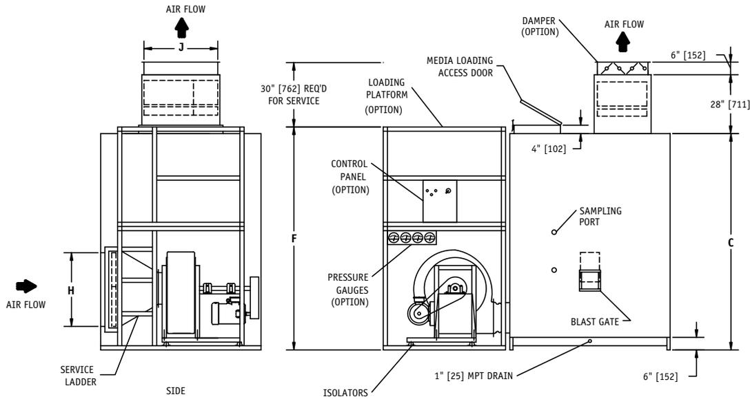
**Vertical Discharge Model - Optional intake filter location (right hand or left hand side)**
